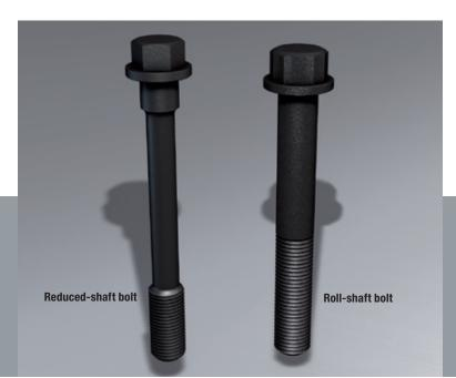
Advantage of stretch bolt: As opposed to a rolled shank bolt, it can be tightened beyond its elastic limit (yield point) into the plastic region — a guarantee for high and uniform bolt clamping forces.
