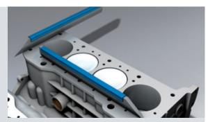
**2.** Use a straightedge to check the surface flatnesses; longitudinally and transversely.
