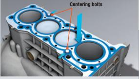
**6.** Position the head gasket accurately on the engine block. Do not use any additional sealing compounds, grease or oil.
