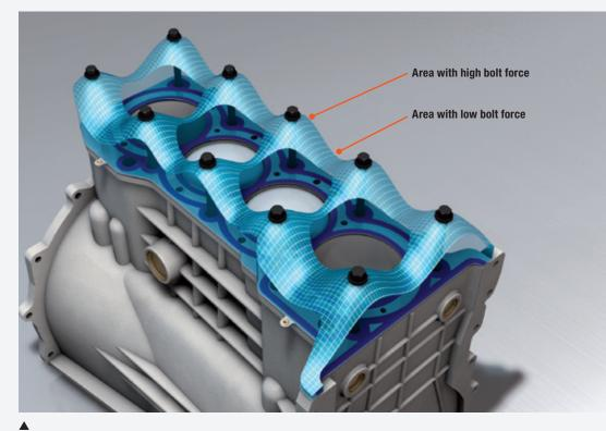
When torquing the cylinder head bolts, the bolt force generates a surface pressure, which is essential for achieving a perfect seal.
