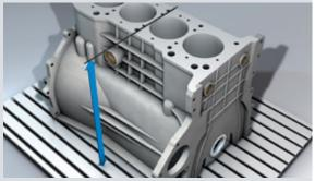
**4.** Observe the minimum dimensions of engine block and cylinder head according to the manufacturer's specifications, as well as the specified head gasket thickness.
