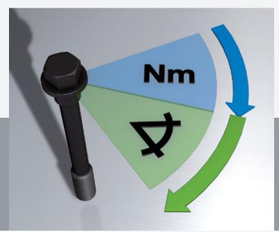
Torque-angle method using pretorque and tightening angle.
