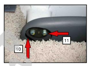
6. Remove the handbrake cover, mark and trim as needed, figure 12.
