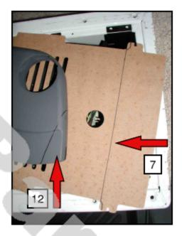
19. Place the small board across the front portion of the pedestal. Following the passenger directions, install the swivel and seat.
