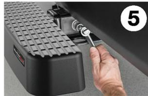
Tighten to a snug fit, do not over tighten (approximately 30-40 ft/lbs of torque.) For plated hardware, use 15/16" socket or wrench. For stainless hardware, use 1/2" hex key.
