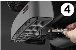
Slide the BumpStep®XL back into your receiver and insert the bolt with lock washer under the head of the bolt, then the flat washer. Flat washer can be eliminated if there is a clearance issue on your vehicle.
