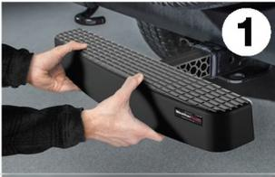
Slide the 2" square portion of your BumpStep®XL into your 2" receiver with the grooved step surface facing upwards.
