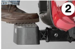
Insert the BumpStep®XL to the hole that allows for enough room to fit just the ball of the foot centered on top with the tip of the shoe clearing the bumper.
